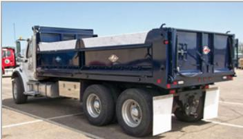
J-Craft's Contractor Medium Duty Dump Bodies offer features you need for the busy season ahead. With heavy duty floors, tailgate, single or split fold sides and a robust structural understructure, the J-Craft Contractor Dump Body was designed and built to handle all the
