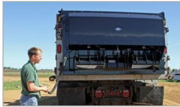
As an added feature, J-Craft's Material Master™ Tailgate, with adjustable opening independently controlled automatic metering gates, allows you to direct material where you need it from the safety of the cab or sides of tailgate. Add versatility and convenience to your heavy
