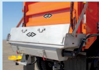
Direct drive design minimizes maintenance and allows independent control of auger and spinner.
