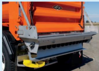
Full opening bottom trough hinged on body side for accessibility and complete clean out.
