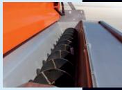
Fully tapered trough eliminates all flat surfaces preventing material hang ups. The boxed in top cover adds strength.
