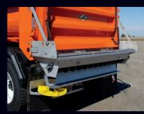
Full opening bottom trough hinged on body side for accessibility and complete clean out.
