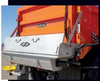
Direct drive design minimizes maintenance and allows independent control of auger and spinner.
